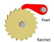
This would be a suitable mechanism for the operation of the turnstile.
