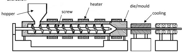
This process is used to produce items of uniform profile such as curtain rails and plumbing pipes. Plastic granules are fed from a hopper through a die by a rotating screw. The plastic is heated in the chamber before it enters the die and cooled by air jets or water as it leaves the die. The extruded products can be cut into lengths or coiled. Thermoplastics such as polythene, PVC and nylon are commonly extruded.
