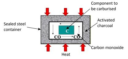
The piece is packed in a box with a carbon rich material such as charcoal and placed in a furnace at 920°C (above UCT). This allows the carbon to diffuse into the piece.
